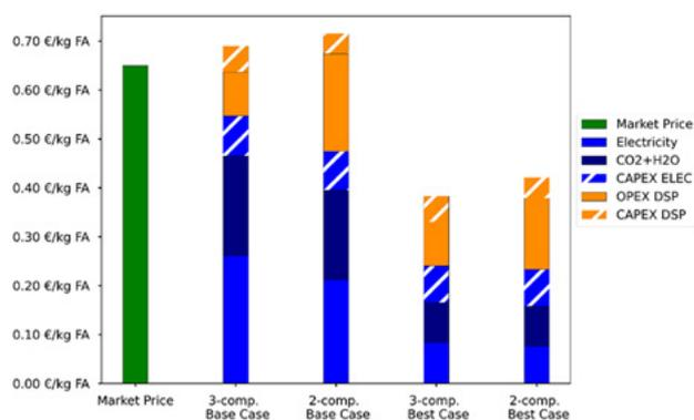
Figure 12: Comparison of the base case with the best case scenarios for both the 3- and 2-compartment process parameters.
