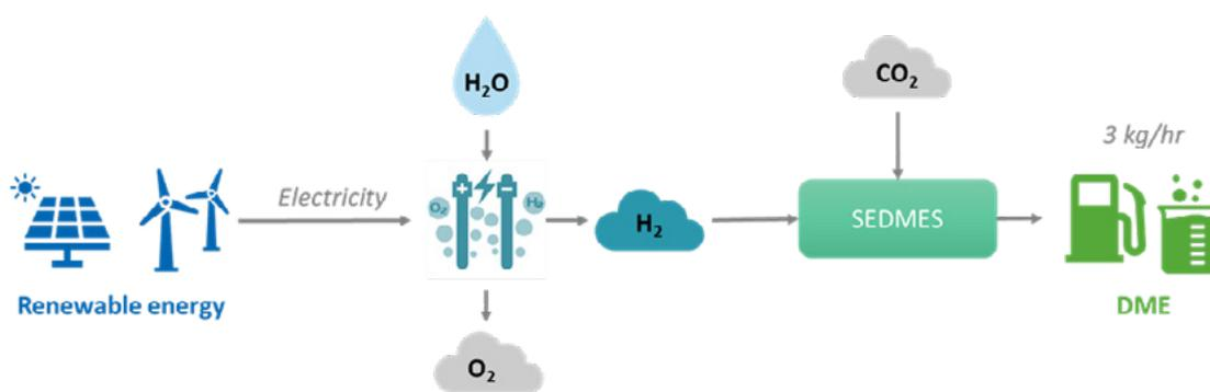
Figure 7: Overview of the envisioned Power-to-X process to convert CO<sub>2</sub> to DME.
