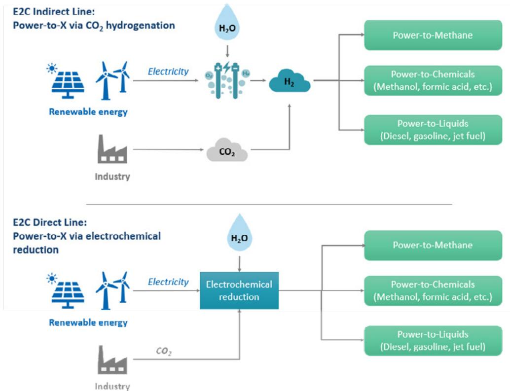
Figure 2 Schematic of Power-to-X via CO<sub>2</sub> hydrogenation (the E2C indirect line) and Power-to-X via electrochemical reduction of CO<sub>2</sub> (the E2C direct line).
