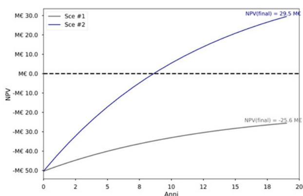
Figure 11: Net present values for two scenarios of CO<sub>2</sub> prices. Case #1: indicative of a positive price for CO<sub>2</sub>. Case #2: the possibility of when the cost of CO<sub>2</sub> emission allowance certificates is significantly increased, therefore Power-to-X SEDMES technology receives money from the CO<sub>2</sub> supplier.
