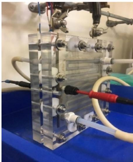
Figure 6 Scale-up of AEM cell (100 cm<sup>2</sup>)
