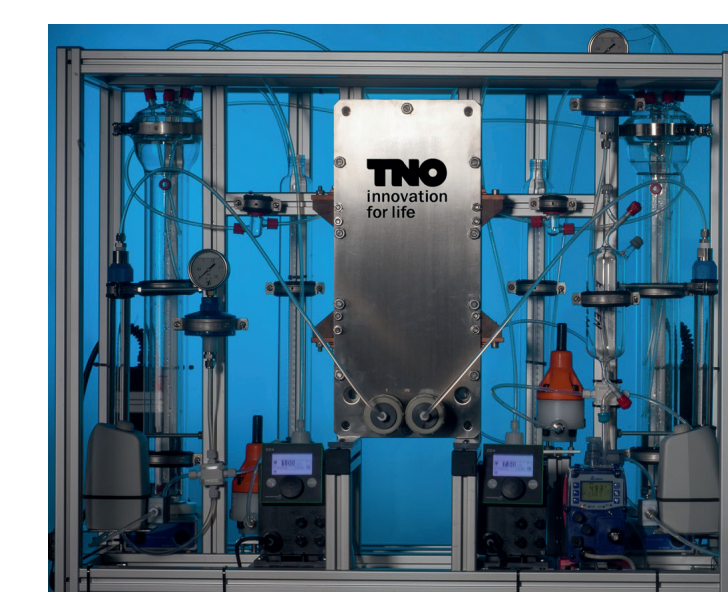
Figure 3. Electrolyzer developed at TNO for continuous synthesis process
