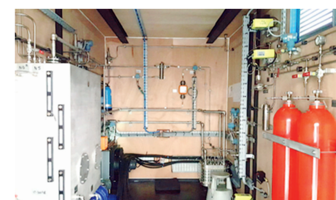
Figure: Prototype 50 kW PEMWE stack and system
