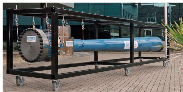
10 kW bench scale electrically driven thermo-acoustic heat pump, which uses waste heat at 50-120 °C to deliver process heat 100-200 °C. Developed by ECN together with Bronswerk.
